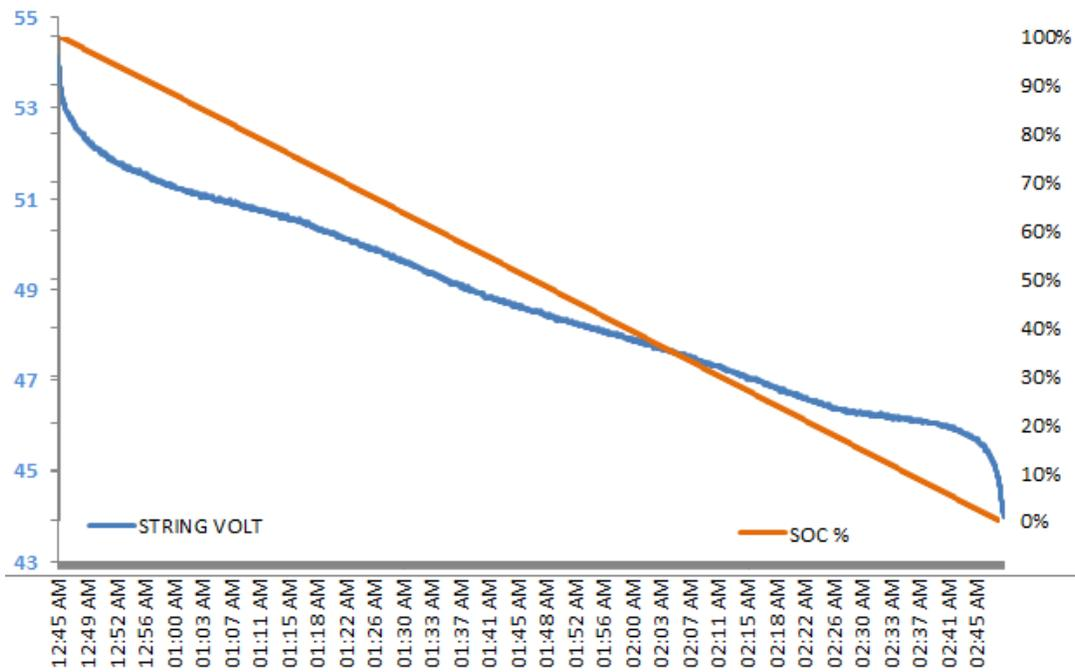
Graph 2: Sirius 7.1kW.h V-SOC curve at 0.5C
